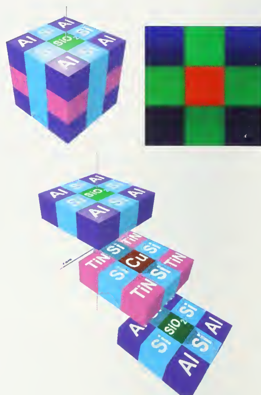
Figure 2. (top left) Phantom sample consisting of a "Rubik's cube" of aluminum, silicon, silicon dioxide, titanium nitride, and copper. This fictional sample contains many of the materials used in modern semiconductor devices, admixed and juxtaposed on the nanoscale to simulate the complexity of true 3D chemical imaging problems. Each of the 27 smaller cubes is 100 nm on an edge, so the entire assembly is 300 nm on an edge. The beam (purple vertical line) is shown striking the sample in the center of the \text{SiO}_2 subcube. (top right) 3-color X-ray elemental map showing quantitatively the detected X-ray intensities for the Cu K\alpha X-ray emission line (red), the Si K\alpha X-ray emission line (green), and the N K\alpha X-ray emission line (blue) after excitation with a 20 keV incident electron beam. Note the differential absorption of the Nitrogen K line from bottom to top (the X-ray detector is off the top of the image) and the bleeding of excitation near the phase boundaries. The X-ray map is 300 nm on a edge. (bottom) The same cube shown with the top, middle, and bottom layers vertically expanded and horizontally translated to reveal the 3D structure more clearly.
